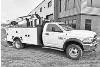
'17 Dodge Ram 5500HD, Cum. 6 cyl., 6.7L dsl., A/C, cruise, pwr. windows, exhaust brake, auto., 7.25F, 13.5R, 10'11" body, manual stabilizers, '17 IMT 2-section crane, stk. #5500 . . . Call
