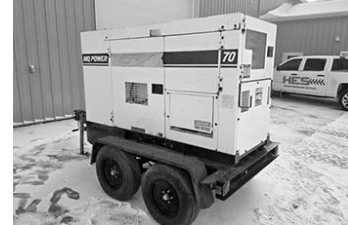
'99 Multiquip Whisperwatt 70 KVA JD 4045TF150C 4 cyl. 90 hp 4.5L dsl. eng., 70kVA/ rated 3-phase output, 480V/240V rated voltage, 40kW rated sgl. outlet, 11,900 hrs., stk. #8897 . . . $12,500
